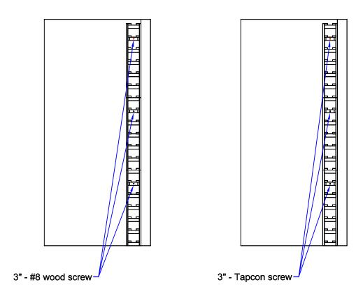
For uneven surfaces, like brick, we recommend using a slotted "L" bracket that you secure to the post with a 5/8" screw and then use a Tapcon screw to secure to the wall.
